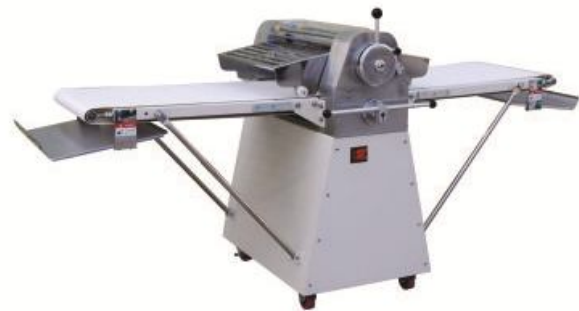
Dough Sheeter - Floor Model Size : 2550x880x1180 Roller Speed : 124 r / min Roller Adjustable Gap : 1-35mm
